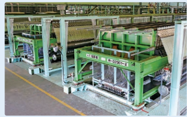
Electrolysis of salt
